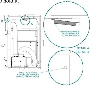
4. Firmly push the faceplate to the fireplace in order to secure the bottom.
