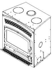
5. Secure the faceplate using the two self-tapping screws provided with the owner's manual.
