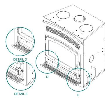
6. Fix the springs of the bottom of the faceplate to the washers on the louver.
