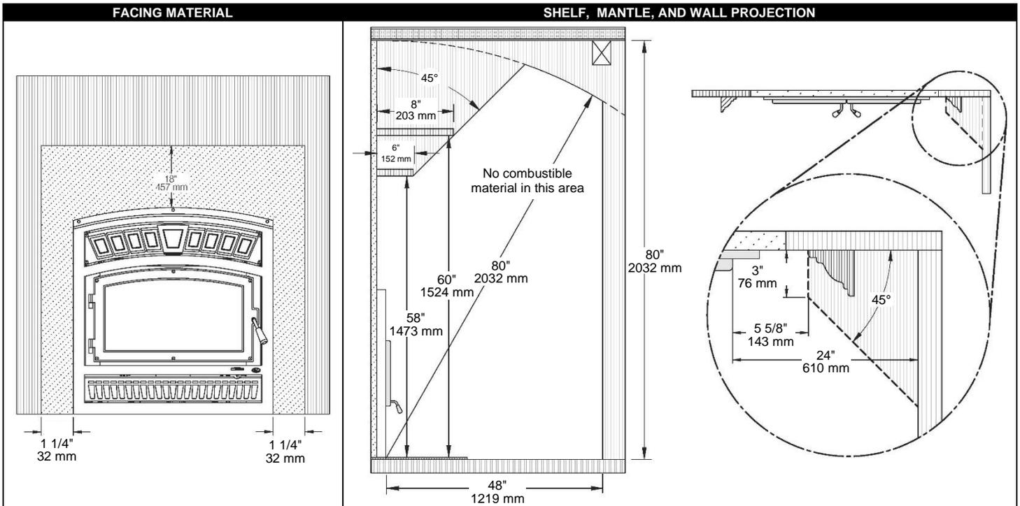
\*If fireplace is installed directly on the floor or on a raised base of less than 4", the hearth extension floor area must extend at least 16" (406 mm) in front of the fireplace with R-value equal to or greater than 1.00. Use 1/2" Micore or refer to manual for equivalent insulation.
